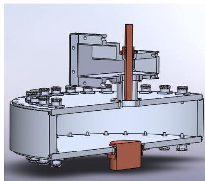
Figure 4: ESRF 1.41 GHz TM030 cavity combiner.
