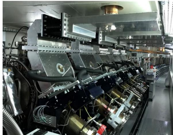
Figure 1: String of five HOM damped 352.37 MHz cavities in the EBS storage ring. Per cavity:  $R/Q = 145 \Omega$ ,  $Q_0 = 35700$ ,  $R_s = 5 M\Omega$ ,  $V_{acc-nom} = 500 \text{ kV}$ ,  $V_{acc-max} = 750 \text{ kV}$ . Longitudinal HOM impedances for 13 cavities remain well below threshold for LCBI [4].
