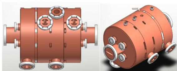
Figure 3: TM020 4-cell harmonic cavity for EBS [11].
