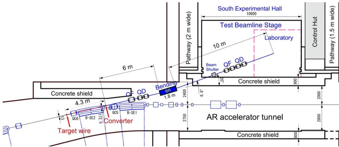
Figure 5: Overall layout of the PF-AR test beamline.
