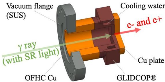
Figure 7: Water cooled Cu converter.
