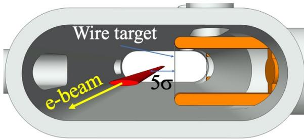
Figure 6: Perspective view of the target wire insertion mechanism.
