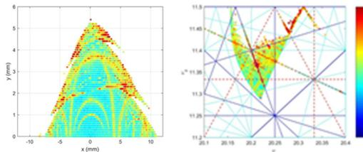
Figure 4: On-momentum FMA at the injection point.
