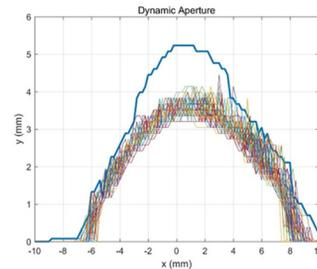
Figure 6: Dynamic aperture at injection point (100 seeds).
