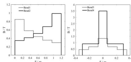
Figure 5: Magnetic field distribution of the dipoles.
