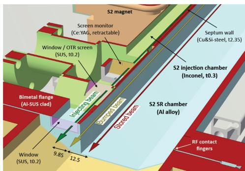
Figure 3: Configuration of the vacuum chamber at the PF ring injection area after modification.
