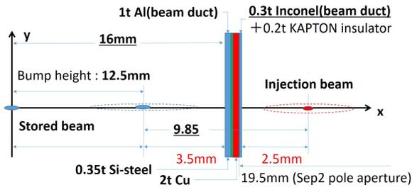
Figure 1: The beam arrangement and septum wall structure at injection point.
