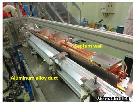
Figure 4: The final setting of beam chambers.
