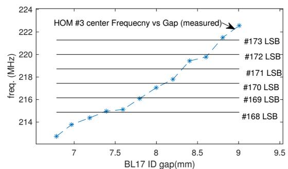
Figure 1: The resonant frequency of the measured HOM #3 crosses different CBI modes with ID gap change.
