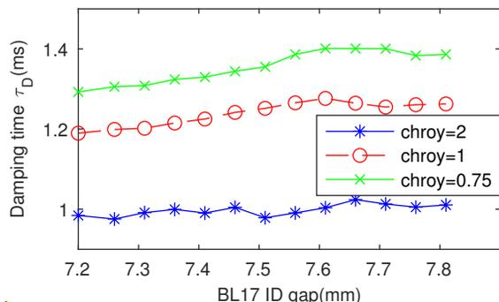
Figure 5: Damping time for CBI mode #168 at different BL17 ID gaps with different  $\xi_y$ .
