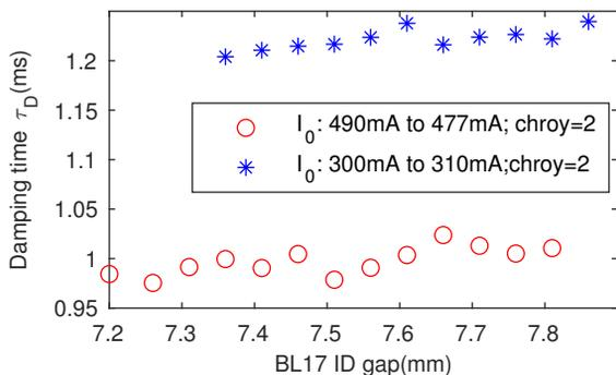
Figure 4: Damping time for CBI mode #168 at different BL17 ID gaps with different stored beam currents.
