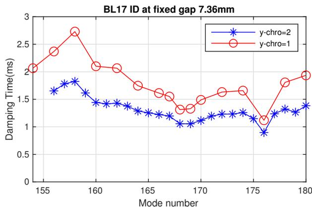
Figure 6: Damping time for different CBI modes while keeping the BL17 gap at 7.36 mm.
