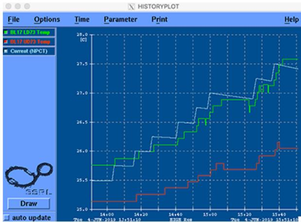
Figure 2: SPEAR3 history plot during BL17 ID beam commissioning shows readings of the TCs on the ferrite dampers.
