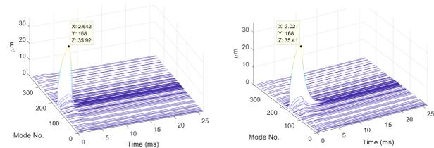
Figure 3: Drive-damp measurements at 7.36 mm gap with the BxB feedback on (left) or off (right) after the drive.
