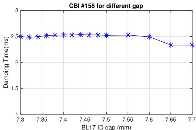
Figure 7: Damping time for CBI mode #158 at different BL17 ID gaps.
