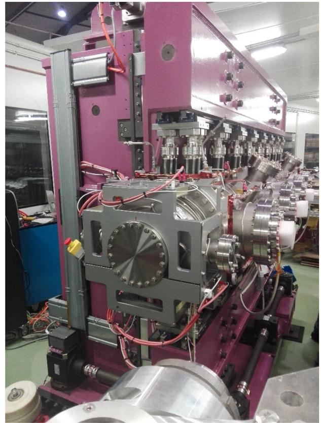
Figure 4: XAIRA undulator after SAT measurements including vacuum, magnetic field and EPS system.
