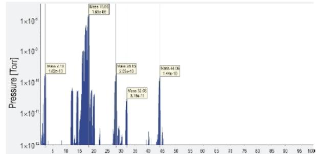
Figure 5: RGA analysis of residual gases in XAIRA vacuum chamber after its closure.
