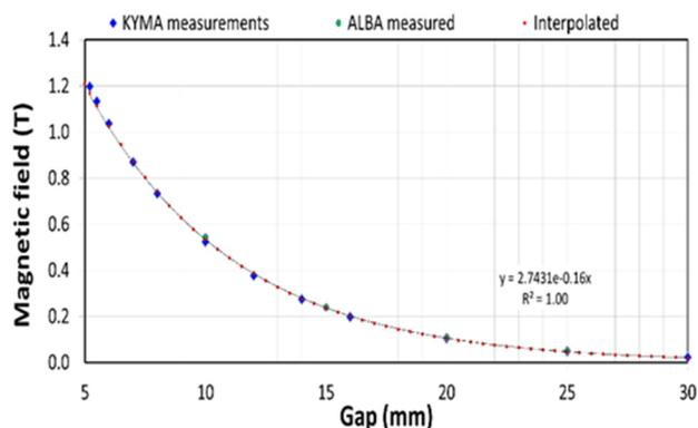
Figure 7: Correspondence between ALBA and KYMA magnetic field vs gap measurements.
