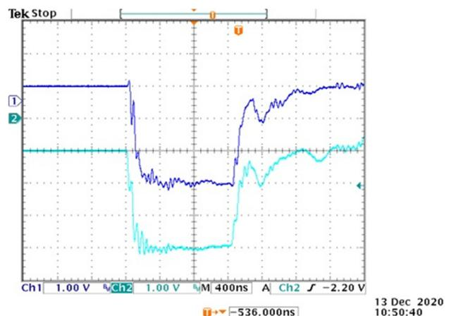
Figure 2: The thyatron switch PFN drive current pulses.
