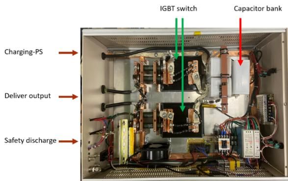
Figure 4: The detailed layout of the IGBT pulser.
