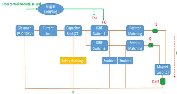
Figure 3: The circuitry layout of the IGBT pulser.
