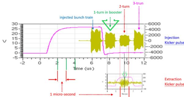
Figure 7: The booser BPM signals for both injected bunch train and the extraction bunch train together with the associated IGBT injection/extraction pulsers.
