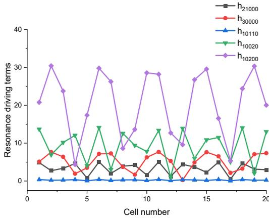
Figure 1: Changes of the third-order resonance driving terms with the cell number.
