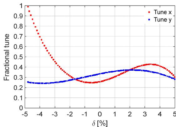
Figure 4: Transverse tune shifts with momentum, tracked for 1024 turns.
