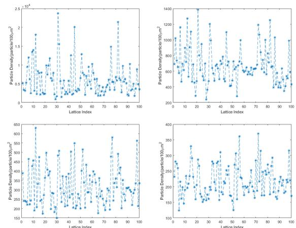
Figure 4: The maximum macroparticle density lost on the collimators. The upper left is the result with no kickers, the upper right is the result with a single horizontal kicker, the lower left is the result with a single vertical kicker, and the lower right is the result with both horizontal and vertical kickers.
