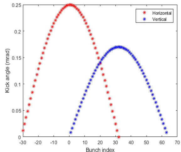
Figure 1: A diagram of kicker waveforms.
