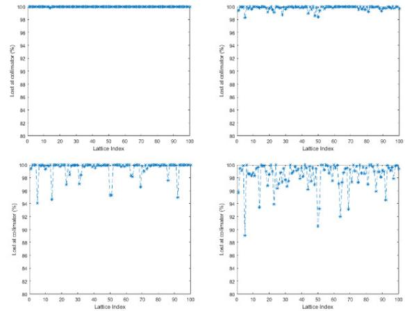
Figure 3: The proportion of particles lost on the collimators. The upper left is the result with no kickers, the upper right is the result with a single horizontal kicker, the lower left is the result with a single vertical kicker, and the lower right is the result with both horizontal and vertical kickers.
