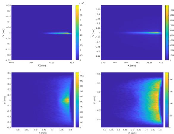
Figure 2: The distribution of macroparticles lost on the collimators under different kicker conditions. The upper left is the result with no kickers, the upper right is the result with a single horizontal kicker, the lower left is the result with a single vertical kicker, and the lower right is the result with both horizontal and vertical kickers.
