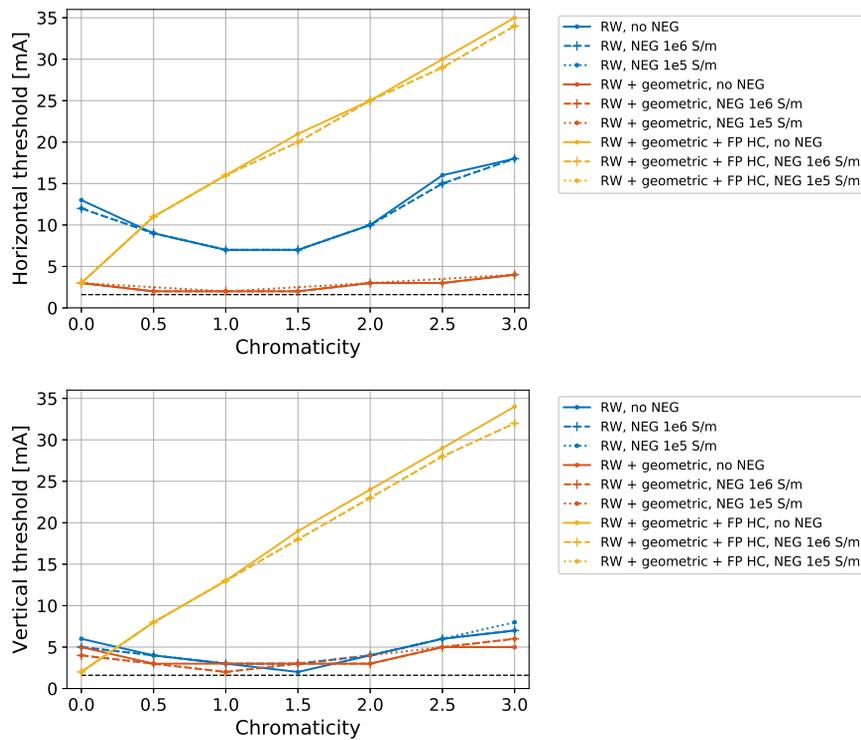
Figure 4: Horizontal (top) and vertical (bottom) threshold currents as function of chromaticity. In these simulations only the transverse impedances have been included. The current requirement for the hybrid bunch is marked (black dashed).
