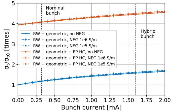
Figure 2: Bunch lengthening compared to the zero current bunch length as function of current including longitudinal resistive-wall, geometric impedance and a third order harmonic cavity set to flat potential conditions. The current requirements for a bunch in uniform fill (nominal) and the hybrid bunch are marked.
