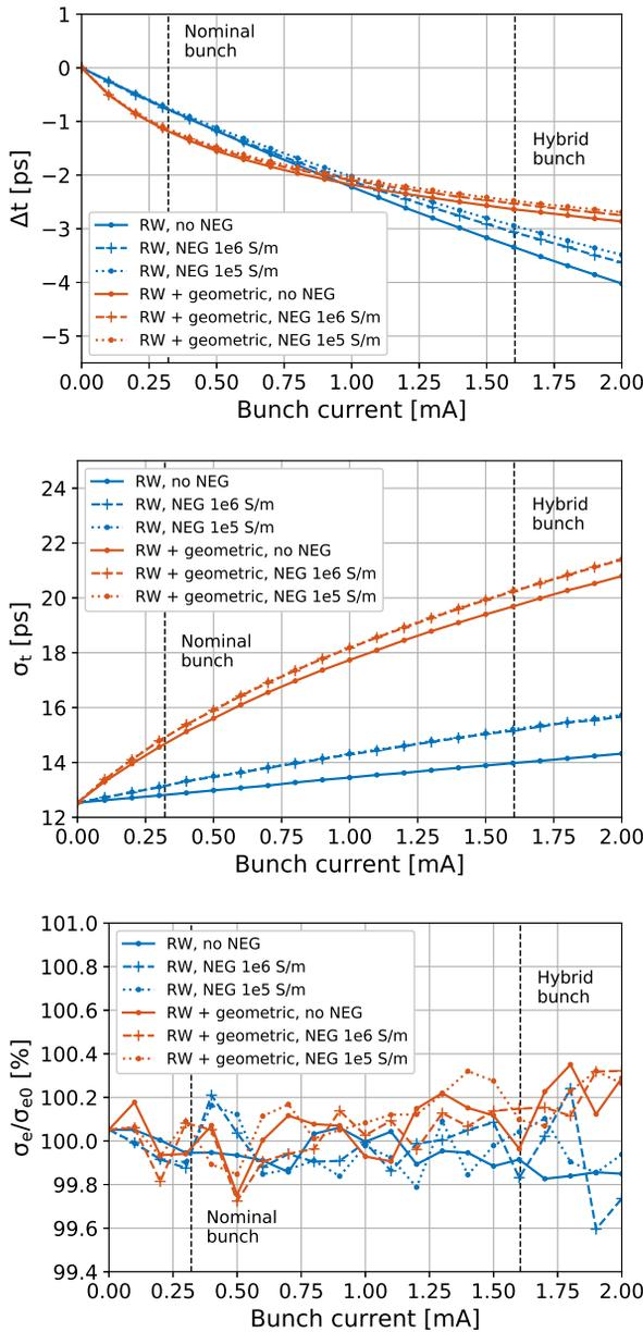
Figure 1: Longitudinal centroid shift (top), bunch length (middle) and energy spread (bottom) as function of bunch current. The bunch current requirements for a bunch in uniform fill (nominal) and the hybrid bunch are marked.
