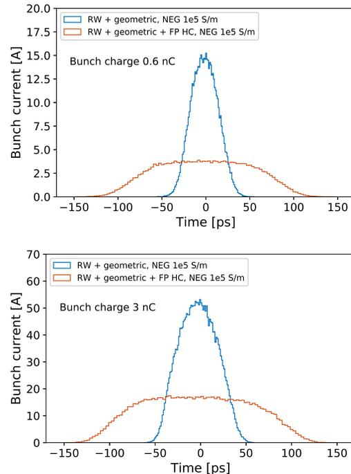
Figure 3: Longitudinal bunch profiles for 0.6 nC bunch (top) and 3 nC bunch (bottom) including resistive-wall (NEG 1e5 S/m), geometric impedance and a third order harmonic cavity set to flat potential condition. In both cases the zero time point corresponds to the zero current synchronous phase.
