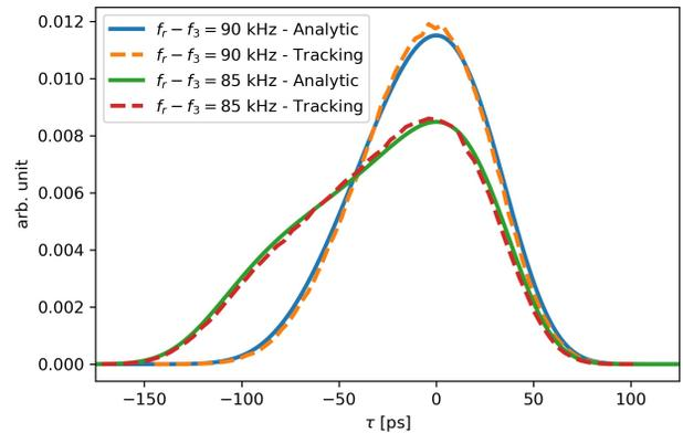
Figure 2: Equilibrium bunch profile for SOLEIL upgrade parameters at 500 mA in uniform filling for two different detunning,  $f_r - f_3 = 85$  kHz and 90 kHz. SOLEIL upgrade parameters can be found in [7].
