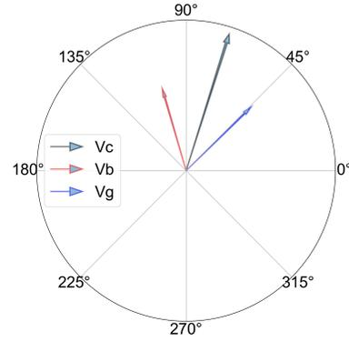
Figure 1: Phasor diagram of the main RF cavity, representing the cavity phasor  $\tilde{V}_c = \tilde{V}_b + \tilde{V}_g$ , the beam phasor  $\tilde{V}_b$  and the generator phasor  $\tilde{V}_g$ .
