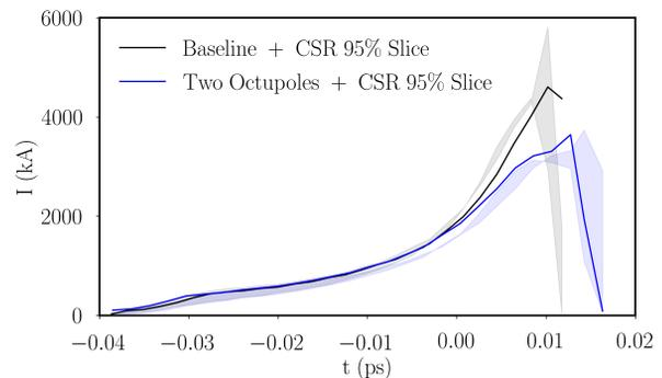
Figure 6: Current profile slice comparison between the original baseline (black) and the dual octupole scheme (blue).
