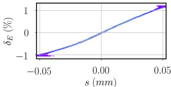
Figure 4: Longitudinal Phase Space evolution of the uncorrected baseline design at the end of BC1.
