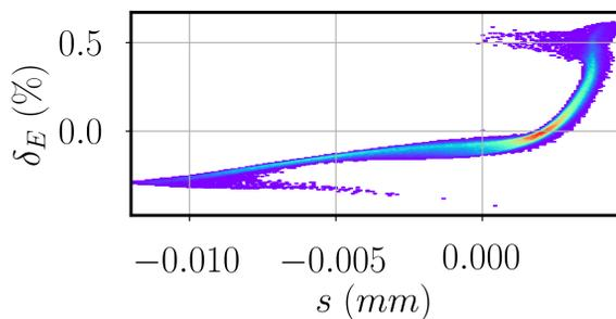
Figure 5: Longitudinal Phase Space evolution of the uncorrected baseline design at the end of BC2.
