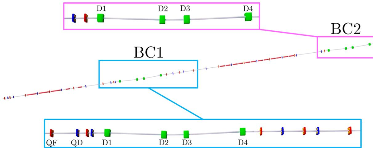
Figure 3: CompactLight Baseline Lattice Design from September 2020 showing the bunch compressors, BC1 and BC2 as indicated. Note, QF denotes the focusing quadrupoles, QD denotes the defocusing quadrupoles. Also note that D1 is the first dipole within the chicane, D2 is the second, D3 is the third and D4 is the fourth dipole within the chicane.
