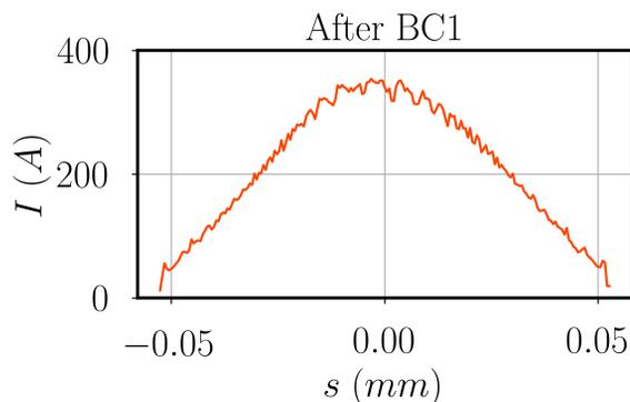
Figure 1: Current Profile of the uncorrected baseline design at the end of BC1.
