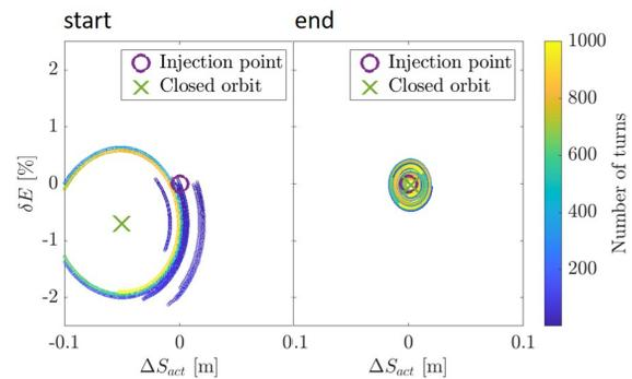
Figure 4: Optimisation of the RF working point as seen in the longitudinal phase space. The starting point (left) shows a poor transmission through the SR (broken blue lines), which is dramatically improved with the new settings (right).
