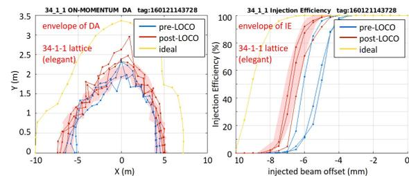
Figure 6: Diamond-II SR DA (left) and IE (right) calculated for an ideal machine (yellow line), for a spoiled machine prior to LOCO corrections (blue lines for 3 error seeds) and after LOCO (red lines). The red shade shows the envelope of 20 seeds calculations done with elegant.
