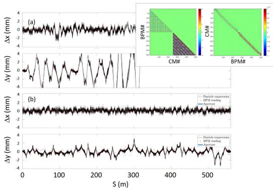
Figure 3: First turn threading in the Diamond-II SR. (Top) initial attempt with total loss of the beam, (bottom) 1<sup>st</sup> turn transmission completed with beam ready for a 2-turn threading. Inset: 1-turn RM and its pseudo-inverse.
