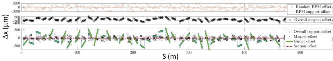
Figure 2: Implementation of errors in the horizontal plane: (top) position errors for the BPMs, (centre) position uncertainty of the magnets, (bottom) motion of girders (green segments), with their clear sway and yaw movements.
