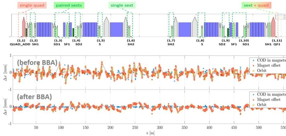
Figure 5: Skew-centring BBA at Diamond-II: (top) pairing between BPMs and magnets, showing BPM to quadrupole (red), BPM to sextupole (green), BPM to two sextupoles and BPM to a quadrupole and a sextupole couplings. (Bottom) effect of BBA seen on the horizontal orbit before and after the procedure, with the final orbit closely following the pattern of misaligned girders.
