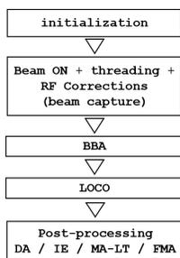
Figure 1: Block diagram representing the sequence of steps used to characterize the commissioning of Diamond-II.
