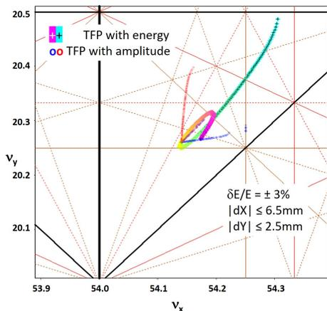
Figure 4: Tune footprint with amplitude (red-blue dots) and with energy shift (magenta-cyan crosses).
