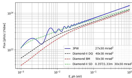
Figure 1: Preliminary study comparing the spectral flux of a 3PW (blue), the present BM at Diamond (red) a DQ element at Diamond-II (black) and for a single dipole (green). Achievable beamline acceptances are currently being clarified.
