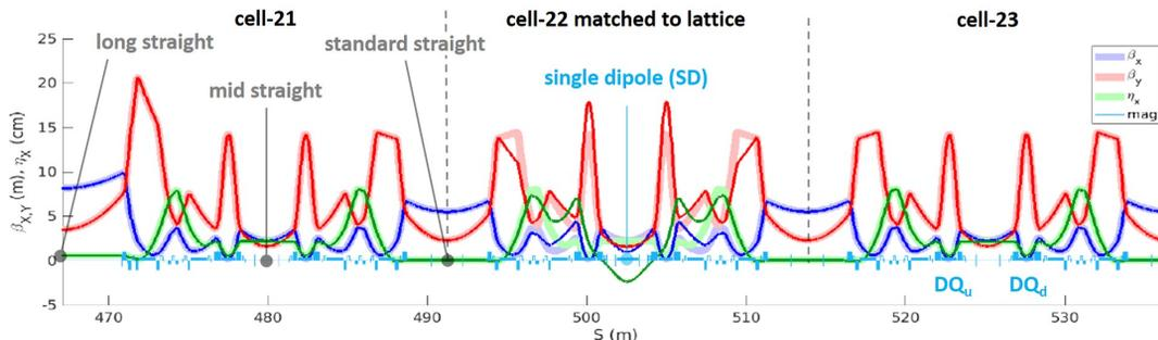
Figure 3: Diamond-II optical functions in the region around cell-22: the light colours illustrate the  $\beta_X$  (red),  $\beta_Y$  (blue) and  $\eta_X$  (green) for the baseline lattice. The dark colours describe the modified lattice, where a bending magnet has been introduced in the mid-straight of cell-22. The superposition of the optical functions outside of cell-22 is testimony of the good matching obtained in the re-design of the lattice.
