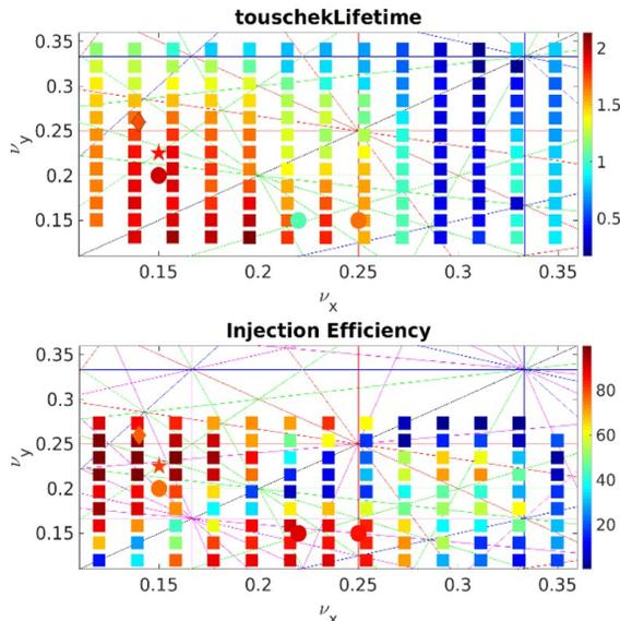
Figure 5: Tune scans to identify the best (LT, IE) for the single dipole lattice. (Top) LT scan, (bottom) IE search.
