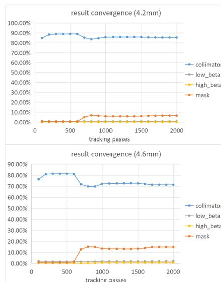
Figure 2: The particle loss ratio versus tracking pass number. (top) 4.2 mm aperture. (bottom) 4.6 mm aperture.
