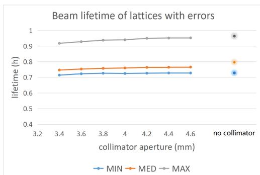
Figure 3: The beam lifetime with respect to different collimator apertures, for the lattices with errors.
