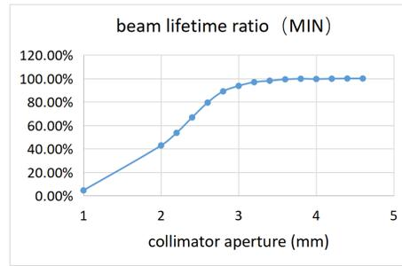
Figure 4: The ratio of beam lifetime with small collimator apertures to that without collimators, for the “MIN” lattice.
