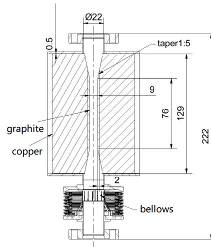
Figure 1: The sectional diagram of the collimator, in which the aperture is 4.5 mm.
