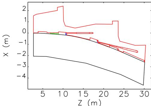
Figure 2: Mid-plane no-go contours for APS-U, showing vacuum and tunnel boundaries.
