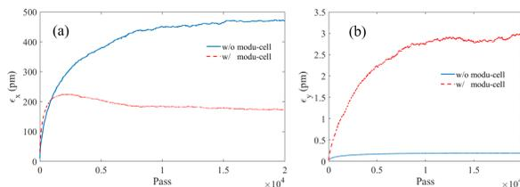
Figure 4: Horizontal (a) and vertical (b) emittance varying with different turns for the case of with and without the modu-cell.
