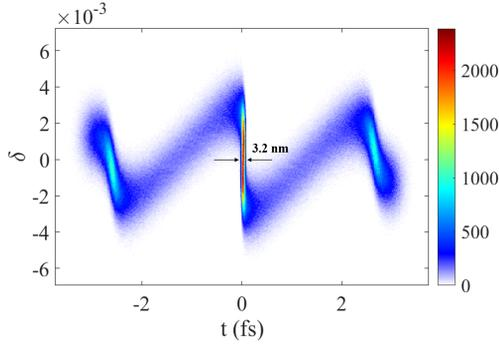
Figure 6: Longitudinal phase-space of the electron beam before enters the radiator.
