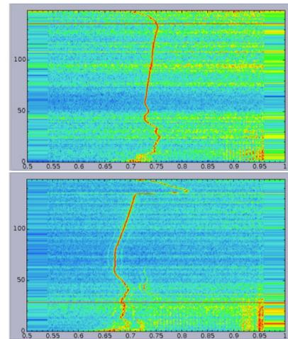
Figure 6: Horizontal (top) and vertical (bottom) tunes for emittance exchange. The vertical tune changes by about +0.1 in 0.7 ms at extraction time (about 140 ms).
