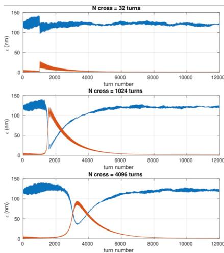
Figure 5: Horizontal and vertical emittance after too fast, optimal and too slow tune crossing.
