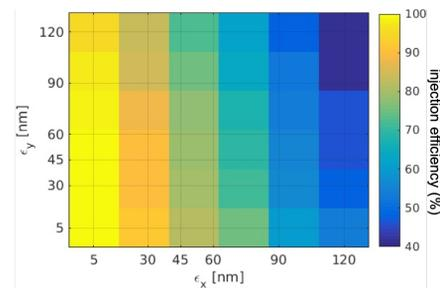
Figure 3: Injection efficiency in the EBS SR as a function of horizontal and vertical emittance of the injected beam.
