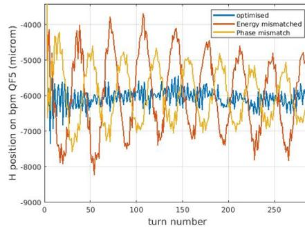
Figure 2: Synchrotron oscillations of the beam entering the booster for three different cases. Blue: optimised, yellow: phase mismatch, brown: energy mismatch.
