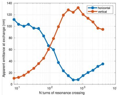
Figure 4: Minimum horizontal emittance and maximum vertical emittance after emittance exchange as a function of duration of the tune crossing.
