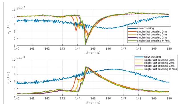
Figure 7: Beam size for different emittance exchange conditions.
