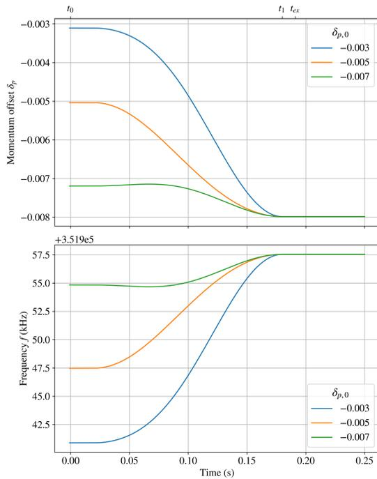
Figure 1: Examples of potential booster frequency/momentum sweeps. The beam is injected at  $t_0$ , the frequency ramp ends at  $t_1$ , and the beam is extracted at  $t_{ex}$
