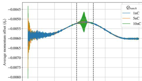
Figure 5: Momentum offset illustrating a frequency bump for bucket targeting. The beam is Robinson unstable between the two dotted lines.
