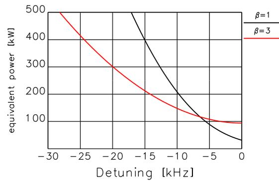
Figure 2: Equivalent power requirements for the booster cavity couplers.
