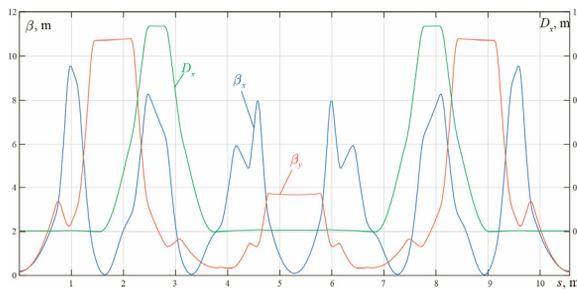
Figure 2: Twiss functions and dispersion.
