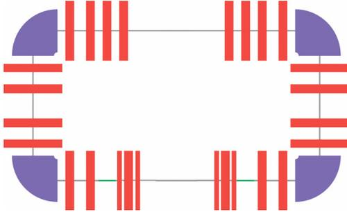
Figure 1: Basic magnet lattice of storage ring.
