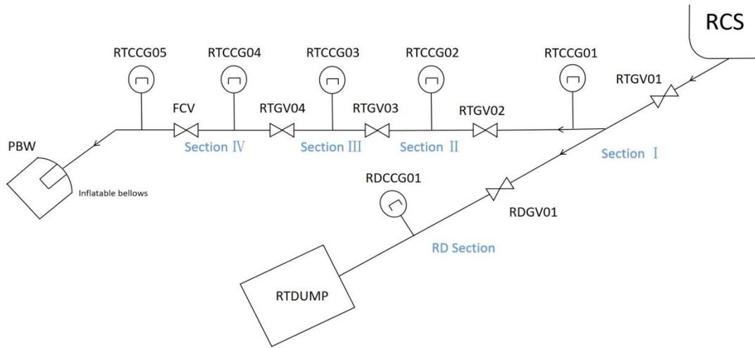
Figure 1: Section of the RTBT (RT: abbreviation of RTBT; GV: gate valve; FCV: fast closing valve).
