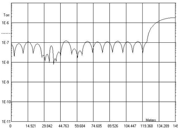
Figure 2: Pressure profile of the RTBT.
