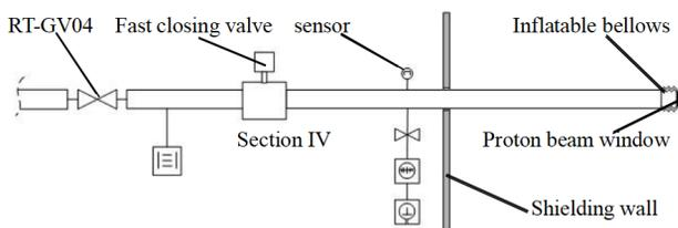
Figure 5: Schematic diagram of fast closing valve system.
