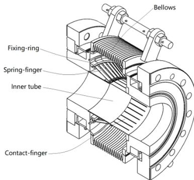
Figure 1: Schematic diagram of the structure of the RF shield bellows.
