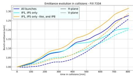
Figure 8: Evolution of the average bunch emittance from the transverse synchrotron light monitors (BSRT) for selected bunch families as explained in the text.
