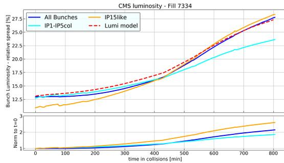
Figure 7: Evolution of the relative spread (rms) of the bunch-by-bunch luminosity for selected bunch families as explained in the text. In the bottom plot the data are normalized to  $t=0$  point to demonstrate the relative increase.
