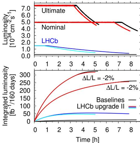
Figure 1: Instantaneous (top) and integrated (bottom) luminosities in black for the HL-LHC baseline and in colours for the LHCb upgrade (red for IP1&5 and blue for LHCb).
