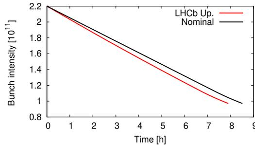
Figure 2: Bunch intensity versus time throughout the fill for bunches colliding in IP1/5 and IP8.
