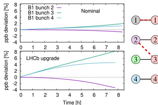
Figure 5: Relative bunch intensity for representative beam 1 bunches with respect to the pair colliding both in IP1&5 and IP8 versus time in the physics fill. Top: Nominal HL-LHC. Bottom: LHCb upgrade to luminosity of  $1.5 \times 10^{34} \text{cm}^{-2} \text{s}^{-1}$ . Right: Collision schemes.
