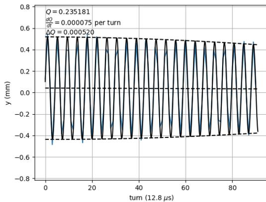
Figure 1: Fitting of the BPM data at injection energy. The resulting tune, tune change per turn and tune spread are indicated.
