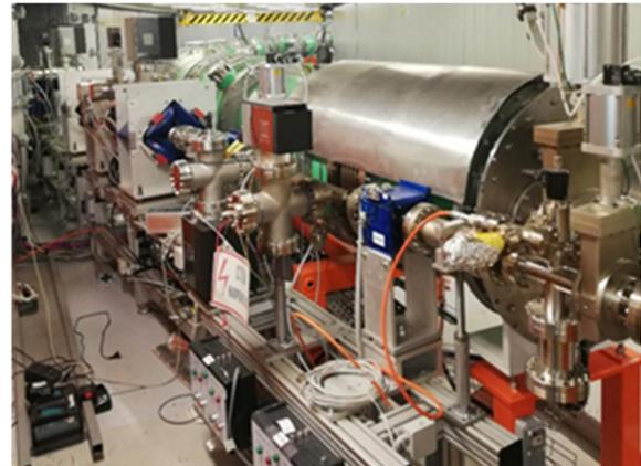
Figure 1: Transport channel HILAC-Booster.
