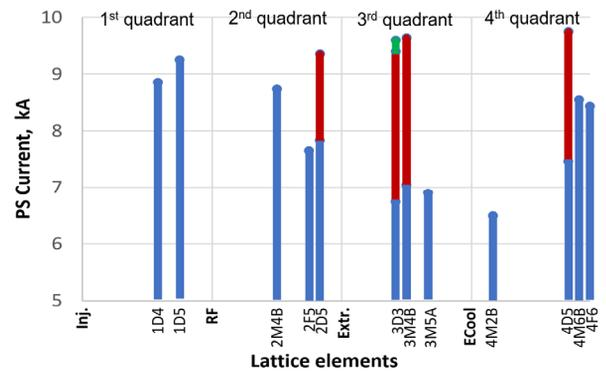
Figure 8: Current amplitude in SC magnetic elements and numbers of detected quenches (blue – first, red – second, green – third one).
