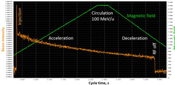
Figure 7: Beam current transformer signal at ion acceleration.
