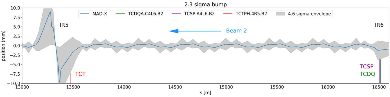
Figure 1: Bump shape computed with MAD-X for a bump strength of  $2.3 \sigma$  at the TCDQ, including a  $4.6 \sigma$  beam envelope. The positions of TCDQ, TCSP and TCTPH are indicated. Beam 2 travels from right to left.
