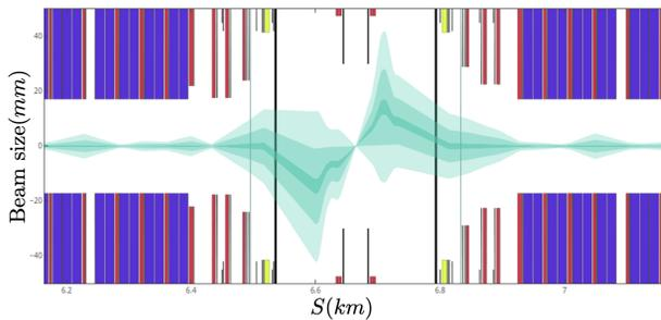
Figure 3: Vertical beam orbit and envelope, expressed in term of beam sigma, shown for 1, 4.7 and 6.7 sigma, at IR1 for the  $\beta^*=15$  cm round collision optics, 5 turns after the onset of the CLIQ discharge in the Q2 magnet.
