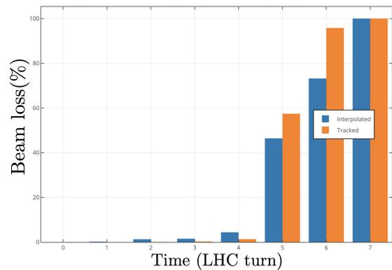
Figure 4: Total recorded losses on a turn-by-turn basis for the spurious discharge of a CLIQ unit at one inner triplet quadrupole. A simplified orbit-excursion model (blue) is compared with a detailed multi-particle simulation (orange).
