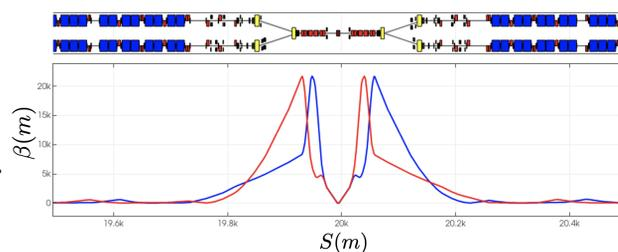
Figure 1:  $\beta$ -functions for the  $\beta^*=15$  cm round beam optics at IR1 (ATLAS). The horizontal (resp. vertical)  $\beta$ -function is shown in red (resp. blue).
