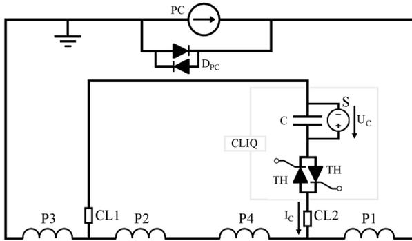
Figure 2: Schematics of a CLIQ system connected to protect a superconducting quadrupole magnet [4].
