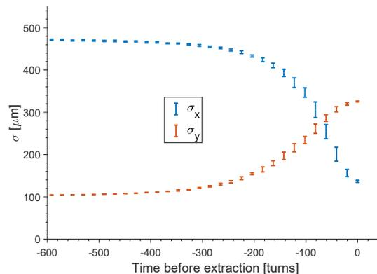
Figure 2: Beam size measurement for various extraction kicker delays on a screen monitor in the SLS booster-to-ring transfer line after applying the vertical beam size minimization.
