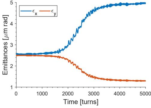
Figure 1: Evolution of emittances while crossing the  $2\nu_x - \nu_y$  coupling resonance with an initial round beam condition. A flat-beam ratio of 3.64 is produced with this configuration.
