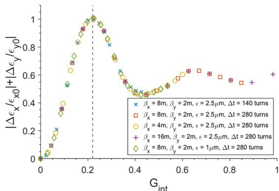
Figure 4: Fractional emittance growth as a function of the integrated resonance strength when pulsing a skew sextupole with working point on the  $2\nu_x - \nu_y$  resonance.
