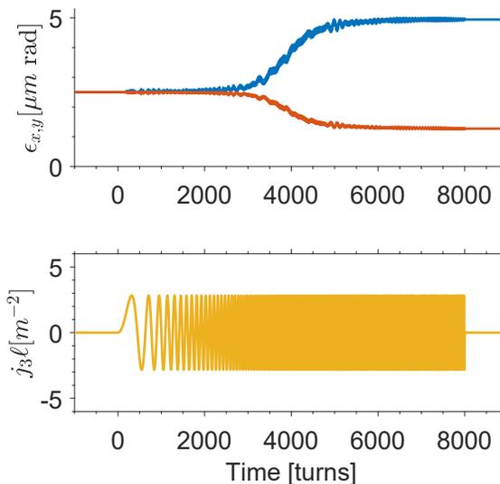
Figure 5: Round-to-flat beam creation using a skew-frequency alternating current skew sextupole. A flat beam ratio of  $\epsilon_x/\epsilon_y \approx 3.9$  can be reached using this method.
