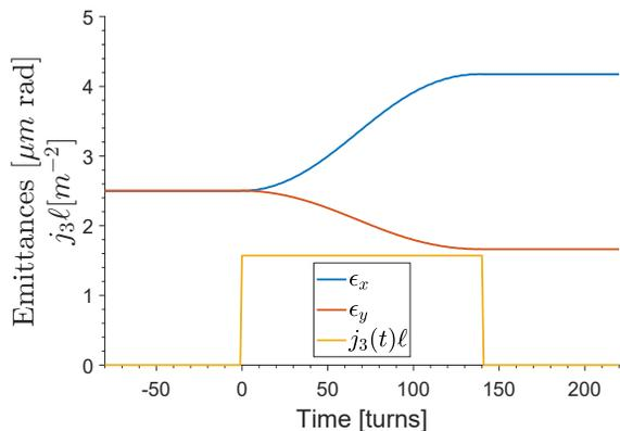
Figure 3: Round-to-flat beam creation using a pulsed skew sextupole on the  $2\nu_x - \nu_y$  resonance. A flat beam ratio of  $\epsilon_x/\epsilon_y \approx 2.5$  can be reached using this method.
