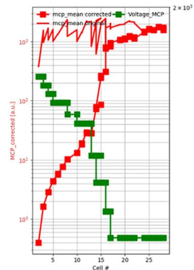
Figure 4: Dependence of the MCP pulse energy signal (red squares) and the MCP voltage (green squares) on the number of active (closed) SASE 2 undulator cells. The uncorrected raw data (red line without symbols) is shown for reference where the MCP gain was changed.
