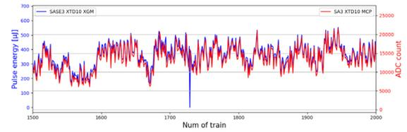
Figure 2: SASE3 FEL pulse energy measured by the MCP and XGM over 6000 consecutive pulse trains.
