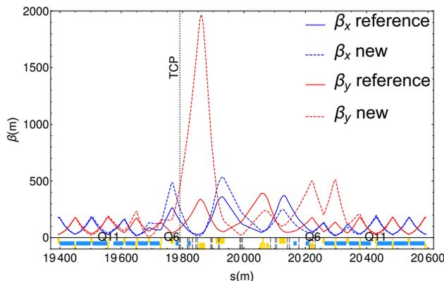
Figure 2: The obtained  $\beta$ -functions in the new optics for beam 1, compared to the reference case.
