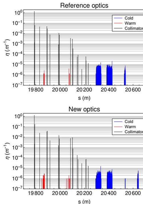
Figure 3: Simulated cleaning inefficiency from SixTrack for the reference and new optics for vertical losses in B1.
