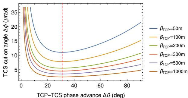
Figure 1: Example of cuts from the TCS on the scattering angle of particles exiting the TCP, as a function of the TCP-TCS phase advance  $\Delta\theta$ , for several different values of  $\beta_{TCP}$ . Typical numerical value for the LHC proton operation have been used:  $n_1 = 6$ ,  $n_2 = 7$ ,  $\epsilon_n = 3.5 \mu\text{m}$ ,  $\gamma_{\text{beam}} = 7461$ . The dashed vertical line shows the optimum phase advance  $\Delta\theta_{\text{opt}}$  from Eq. (2).
