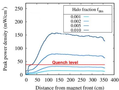
Figure 3: Peak power density in the coils of the Q4 magnet (IR6) for a 0.2 h beam lifetime in HL-LHC. Results were normalized to different halo fractions  $f_{IR6}$ .
