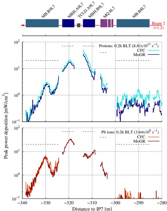
Figure 2: Radially-averaged peak power deposition [mW/cm<sup>3</sup>] in the cold DS magnet coils along beam 1 for protons (top) and Pb ions (bottom) with 0.2 h BLT, comparing the use of CFC and MoGR collimators. Dashed lines indicate the respective estimated magnet quench levels.
