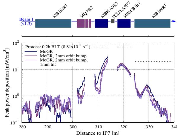
Figure 3: Radially-averaged peak power deposition [mW/cm<sup>3</sup>] in the cold DS magnet coils along beam 1 for protons with 0.2 h BLT, comparing the cases without an orbit bump and a 2 mm orbit bump with and without an additional 1 mm shift. Dashed lines indicate the respective magnet quench levels.
