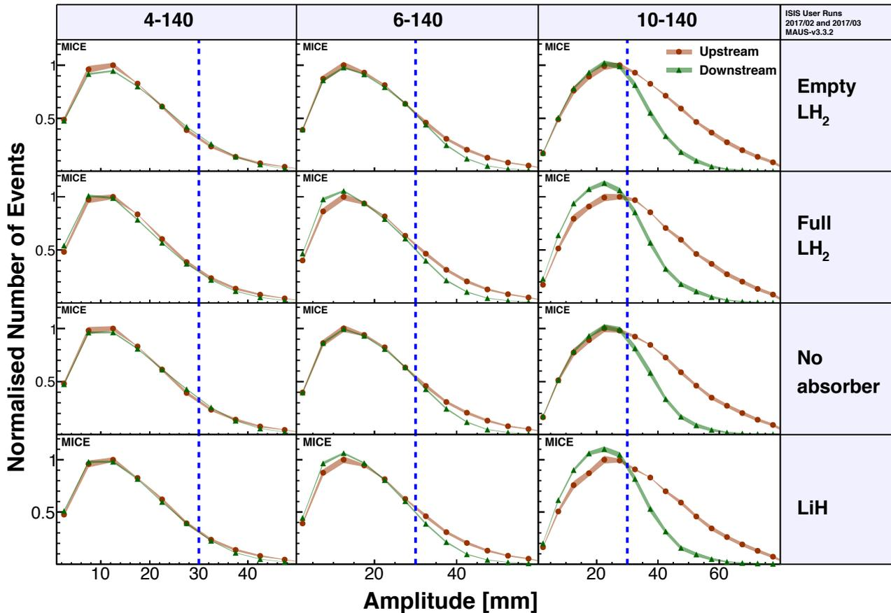
Figure 2: The amplitude distribution of the muon beam upstream and downstream of the absorber for a number of different configurations.
