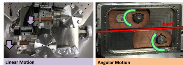
Figure 10: Sirius scraper design minimizes beam coupling impedance. It is based on a special round blade geometry with angular motion driven by a linear-to-angular transmission.
