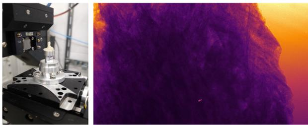
Figure 2: First X-ray microtomography of a carbonate rock sample obtained on Dec.16<sup>th</sup> 2019 at beamline MOGNO, using white X-ray beam from 8 keV to 200 keV from the 3.2 T superbend permanent magnet dipole source. The image was obtained two days after storing the first beam with on-axis injection.
