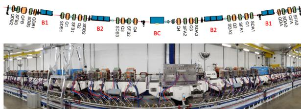
Figure 5: View of Sirius magnets in one 5BA arc.
