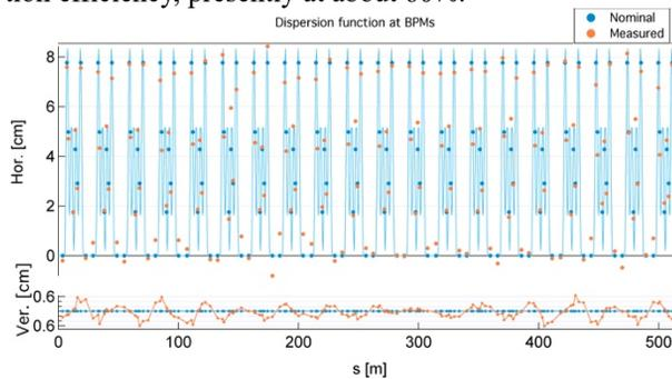
Figure 4: Measured dispersion function along the storage ring as compared to the nominal after correction of dipole calibration error.
