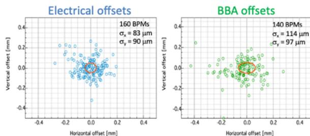
Figure 8: Measured BPM electrical and BBA offsets.
