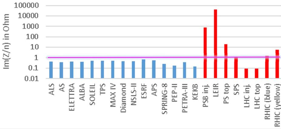
Measured transverse impedance  $\text{Im}(Z_y)$
