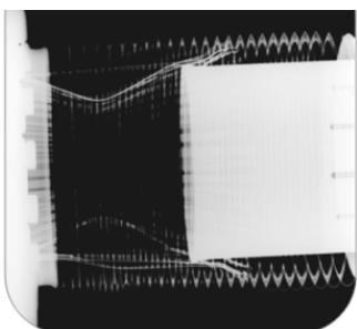
Non-conform: damaged by RF heating from beam
