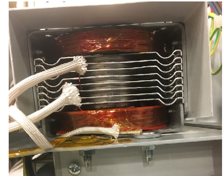
Modified YJ1540 (2M137) with 2X360 turns of trim-coil pancakes, data taken as May, 2019
