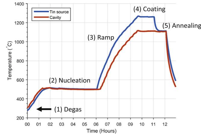
"Wuppertal" configuration, i.e., with secondary heater for the tin source
