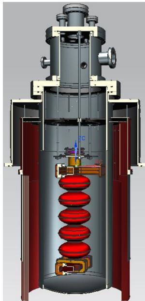
"Siemens" configuration, i.e., no secondary heater for the tin source
