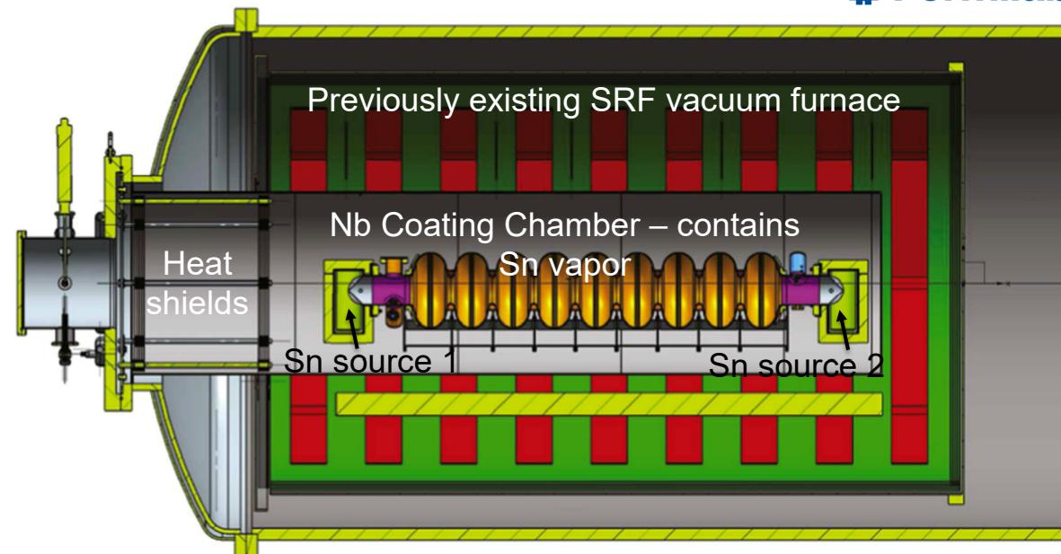
"Wuppertal" configuration, i.e., with secondary heater for the tin source
