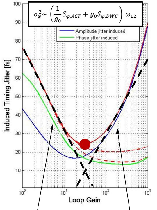
Actuator chain ← → Field detector
