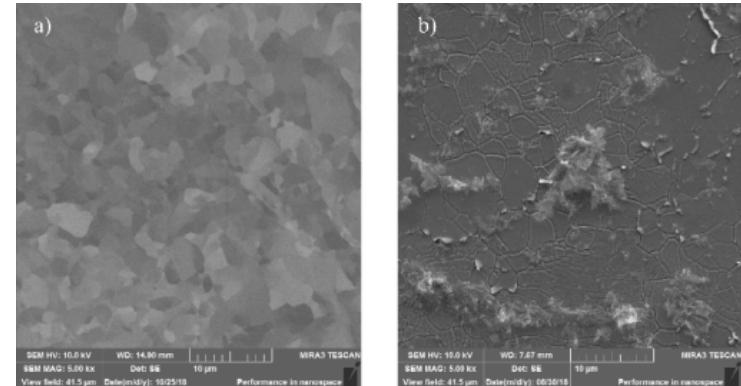
SEM images of the tungsten sample before (a) and after (b) laser accelerated proton irradiation.
