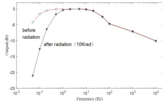
response of semiconductor sensors corresponding to different frequencies
