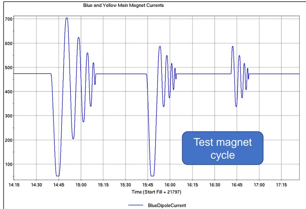
Hysteresis cycles: extra “wiggles” intended to reduce amplitude of persistent current drift, and minimize sextupole component in main dipole magnets
