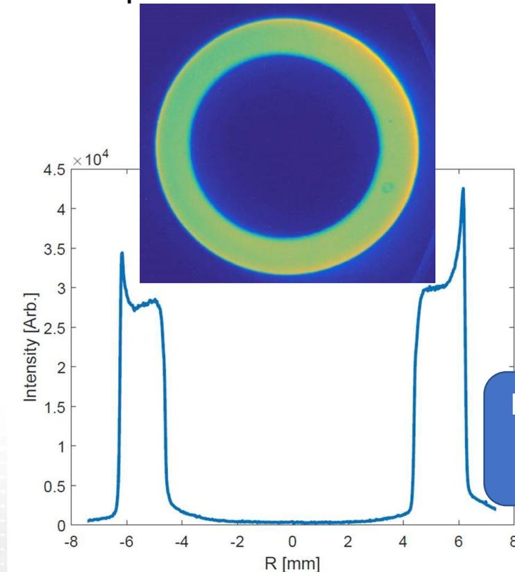
Electron lens collimation study: create hollow electron beam around ion beam
