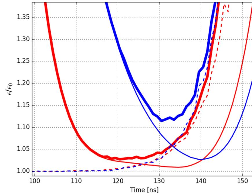
As a result, one can calculate the vertical emittance growth incurred on a bunch by its own injection, as well as the injection of the subsequent bunch (above).
