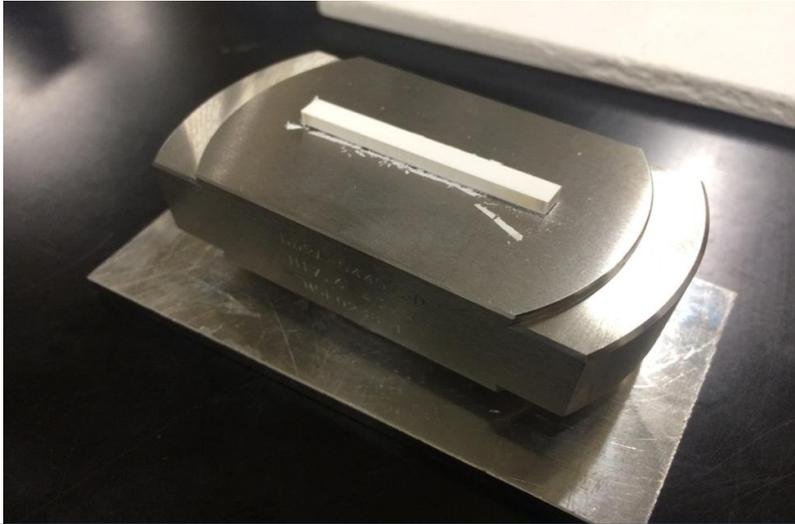
Part of sintering process at RIKEN to form solid  $\text{ZrO}_2$  targets for EBIS. Image courtesy of RIKEN
