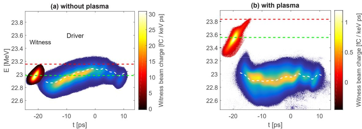
Figure 1: Longitudinal phase spaces of driver and witness bunches measured without (a) and with (b) a plasma of  $(1.2 \pm 0.4) \times 10^{13} \text{ cm}^{-3}$  electron density. The witness bunch ( $t \approx -20 \text{ ps}$ ) was measured with a different camera gain than the driver. Dashed lines indicate witness mean (green) and maximum (red) energies and the driver mean slice energies (white).
