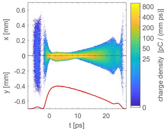
Figure 2: Charge projection in x-t (top) and y-t (bottom) planes for 700 pC double triangular driver and Gaussian witness bunches at the PITZ plasma cell entrance simulated with ASTRA [35]. The normalised bunch current profile is shown in red.
