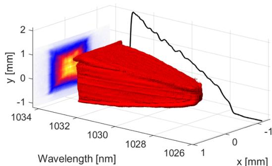
Figure 3: Three-dimensional envelope (red) of a laser pulse shaped to a triangular longitudinal profile (black line) with the SLM-based pulse shaping setup at PITZ, measured in the frequency domain. The intensity was kept constant within every longitudinal slice, while the transverse size is increased gradually. The rectangular transverse projection of the pulse is shown on the left.
