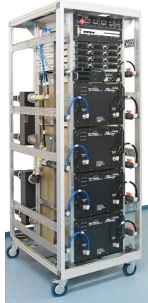
Figure 4: 20 kW amplifier used for conditioning and testing of the couplers.
