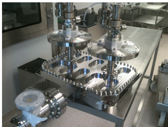
Figure 3: Two couplers fixed on their conditioning box.
