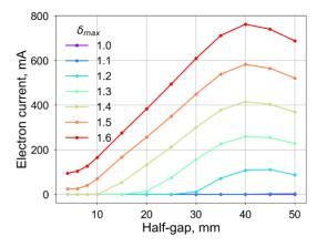
Figure 3: Total electron current in the TDIS as a function of the half-gap for different  $\delta_{max}$  values.
