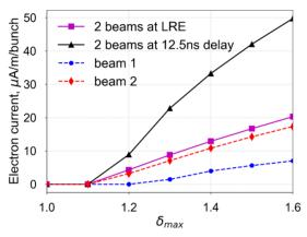
Figure 2: Electron current versus  $\delta_{max}$  at a section of the TDIS with 2 beams delayed by 0 ns (magenta, squares) and 12.5 ns (black,triangles), for beam 1 alone (blue dashed, dots) or beam 2 alone (red dashed, diamonds).
