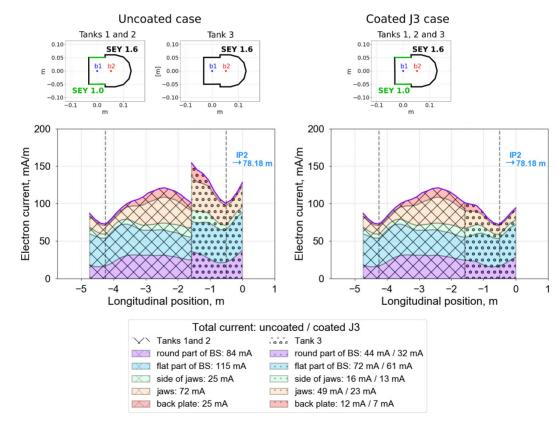
Figure 5: Top:  $\delta_{max}$  configuration for two simulated scenarios. Bottom: contributions to the total electron current from different surfaces in the TDIS for "the uncoated" (left) and "the coated J3" (right) scenarios. The configuration with 40 mm half-gap is considered.
