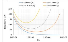
Figure 10: Input power requirement for electron beam of 5 GeV energy and 3.5 A current.
