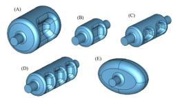
Figure 2: Crabbing cavity geometries considered for JLE-IC. (A) 476.3 MHz Single Cell RFD Cavity, (B) 952.6 MHz Single Cell RFD Cavity, (C) 952.6 MHz 2-Cell RFD Cavity, (D) 952.6 MHz 3-Cell RFD Cavity, and (E) 952.6 MHz Squashed Elliptical Cavity.
