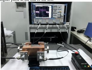
Figure 1: Half structure RF test.
