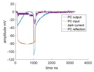
Figure 6: Pulse Compressor(PC) waveforms.
