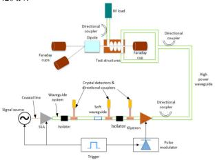
Figure 4: Tsinghua X-band high power test facility layout.
