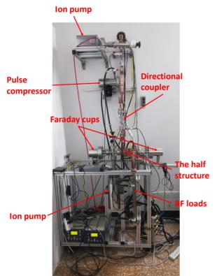
Figure 5: The half structure under test.
