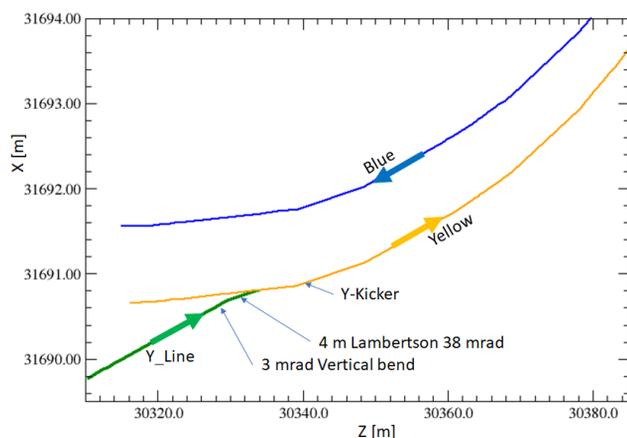
Figure 2: The green, yellow, and blue, traces are the "RHIC survey coordinates" at the entrance and exit of the elements which comprise the Y-Line (green), part of the Yellow ring (yellow) and part of the Blue ring (blue). The location of the 3 mrad vertical bend, the Labmertson septum magnet, and the 1.7 mrad vertically bending Y-kicker is shown on the figure.
