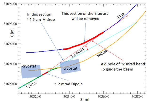
Figure 5: A schematic diagram of the Y-line injection region which helps visualize the steps required for the modification of the beam lines in this region as described in the text.
