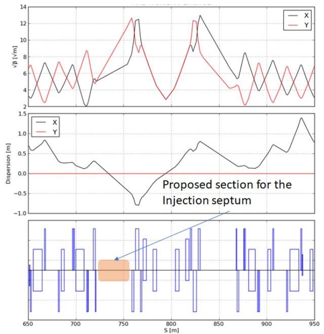
Figure 9: The beta  $\beta_{x,y}$  and the dispersion  $\eta_{x,y}$  functions (top plots) and the placement of the elements at the 4 o'clock region. The highlighted region being the proposed injection region where the dipole and the injection septum magnet will be placed as discussed earlier in the text.
