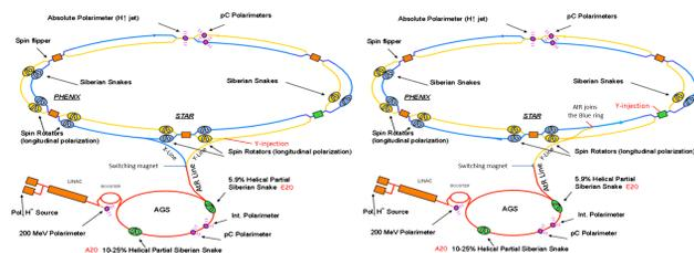
Figure 1: Schematic diagram of the RHIC collider. (left) The AGS to RHIC (AtR) transfer line is located between the AGS and RHIC rings. The switching magnet of the AtR line deflects the beam into either the X-line for Blue ring injection or the Y-line for Yellow ring injection. (right) the Y-line will be extended to join the Blue ring which will transport and inject the beam at IP4 point of the Yellow ring. The X-line which is now part of the AtR line will be eliminated.
