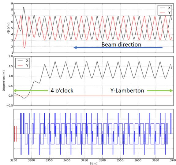
Figure 7: Beam optics of the Blue ring section from the Lambertson magnet to the 4 o'clock IP. From top to bottom plotted are the beta ( $\beta_{x,y}$ ), eta ( $\eta_{x,y}$ ) functions and the location of the elements along the Blue ring.
