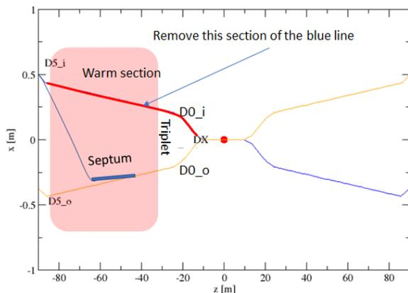
Figure 8: (left) Schematic diagram of the beam injection scheme for the 4 o'clock region. A dipole magnet following the D5-i magnet will guide the beam into an injection septum magnet. The right picture is a rather accurate layout of two possible arrangements of the dipole and septum magnet.
