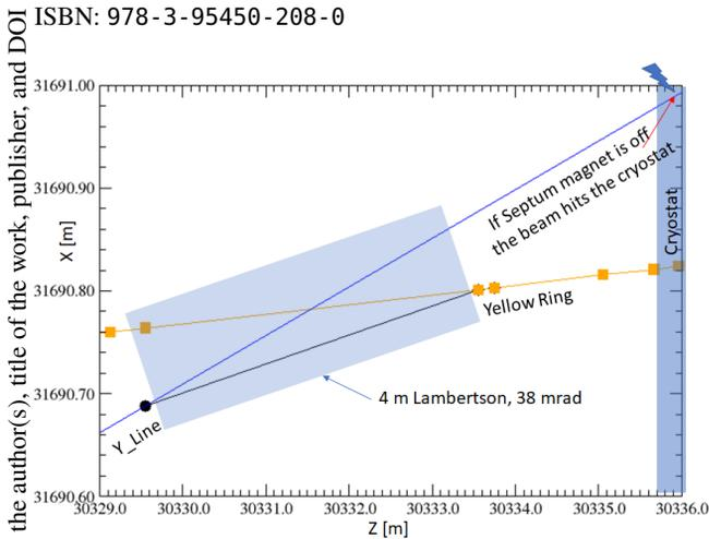
Figure 3: Same as Fig. 2 above but a closeup view showing the survey coordinates at the location of the Lambertson septum magnet.
