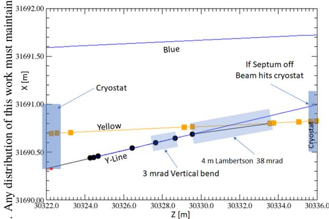
Figure 4: An expanded view of Fig. 3 showing the survey coordinates of devices upstream of the Lambertson septum magnet. The picture on the left of the figure shows that the vacuum pipe of the Y-line is gouging the cryostat of the Yellow arc.
