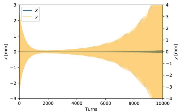
Figure 3: Vertical and horizontal bunch centroid position versus turn number after injection at 6 GeV for the bare Q40 optics and  $Q'_{x,y} = +1$ , at  $N_b = 2 \times 10^{10}$ .
