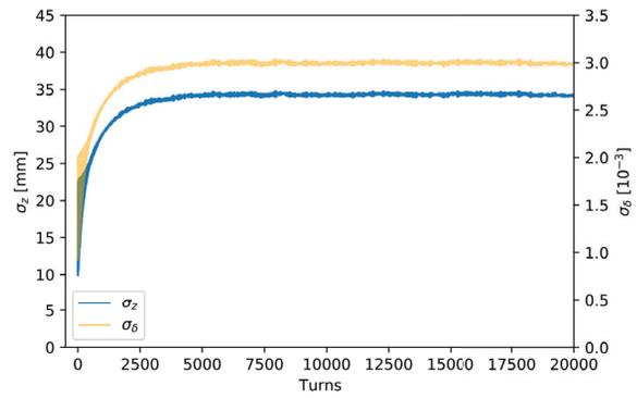
Figure 2: Electron rms bunch length and energy spread versus turn number after injection at 6 GeV for the Q40 optics with additional wigglers.
