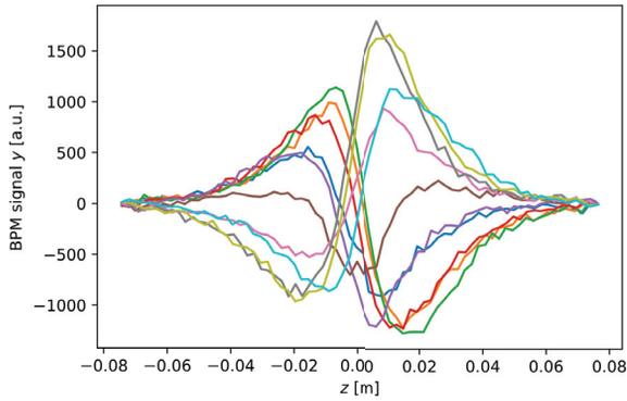
Figure 4: Vertical charge-weighted slice position along the bunch on the last ten turns of the simulation after injection at 6 GeV for the bare Q40 optics and  $Q'_{x,y} = +1$ , at a bunch population of  $N_b = 2 \times 10^{10}$ .
