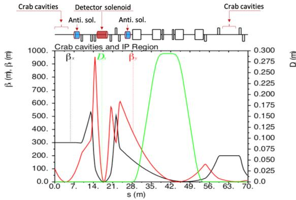
Figure 4: Electron collider ring interaction region optics.
