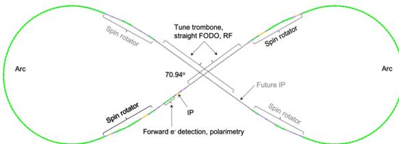
Figure 6: Electron collider ring top-view layout.
