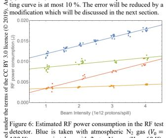
Figure 6: Estimated RF power consumption in the RF test detector. Blue is taken with atmospheric  $N_2$  gas ( $V_0$  = detector. Blue is taken with atmospheric  $N_2$  gas  $(v_0 - 2 \pm 120 \text{ V})$ , orange is taken with 2-atm  $N_2$  gas  $(V_0 = 60 \text{ V})$ ,  $\stackrel{\text{deg}}{=}$  green is tanek with 2-atm dry air ( $V_0 = 120 \text{ V}$ ), and red is Example 1 taken with 1-atm He gas  $(V_0 = 120 V)$ .
