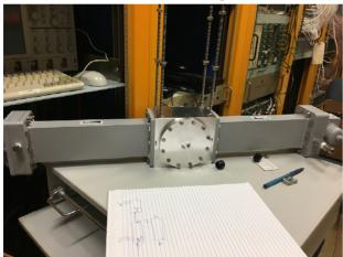
Figure 1: 2.4 GHz RF beam test detector.
