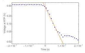
Figure 3: Observed time constant in the RF test detector.
