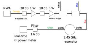
Figure 2: Schematic of RF electronics for the beam test.
