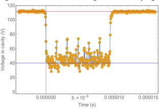
Figure 4: 1-atm N<sub>2</sub> gas-filled RF signal of a six-batches of the 120 GeV/c MI proton beam.
